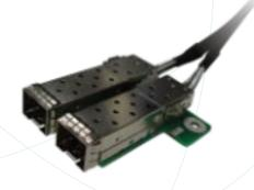
SFP OverPass™ products help avoid high speed signaling through the PCB by creating a direct low loss connection between the ASIC and the external IO port. This helps to enable 28G and 56G hardware system designs, with a roadmap to future 112G and 224G solutions. Using these solutions results in lower signal loss, less PCB design complexity and reduced PCB and signal recovery costs. Fully compatible with SFP industry standards.
